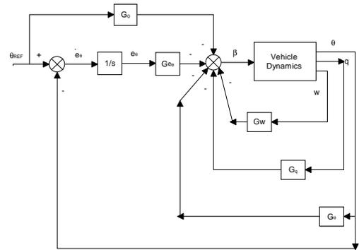
Figure 1 - block diagram of the vehicle with the basic control law.
