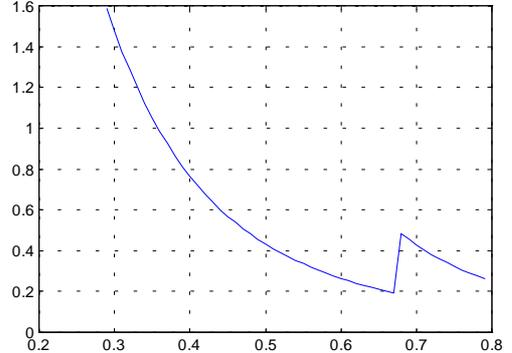
Figure 10 - Time history for the control rate effort  $\dot{\beta}_z$  for the vehicle with the IFD system, 30% uncertainty in  $U_0$  and 30% in  $M_w$  during the transition phase.
