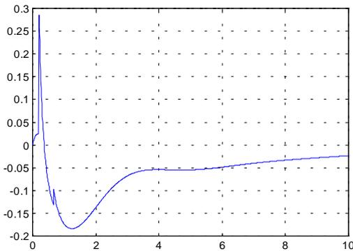
Figure 7 - Control effort ( $\beta$ ) response for a 0.1 step in reference pitch-attitude ( $\theta_{ref}$ ) for the vehicle with the IFD system.
