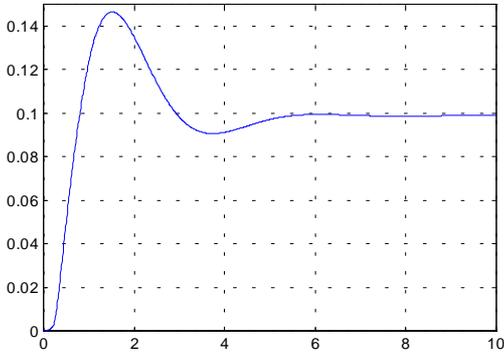
Figure 5 - Pitch-attitude time history for a 0.1 step in reference pitch-attitude ( $\theta_{ref}$ ) for the vehicle with the IFD system.
