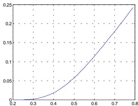
Figure 12 - Time history for the decision function  $\eta_1$  for the vehicle with the IFD system, 30% uncertainty in  $U_0$  and in  $M_w$
