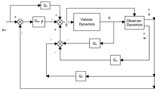
Figure 3 - Observer based control law  $\beta_{z2}$  for observer no.2 - This control law is used when pitch-attitude sensor or normal velocity sensor has failed.
