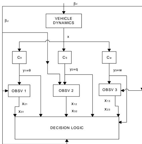
Figure 2 - IFD diagram to be implemented into the onboard computer.
