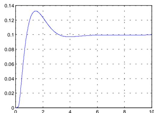
Figure 4 - Pitch-attitude time history for a 0.1 step in reference pitch-attitude ( $\theta_{ref}$ ) for the vehicle without the IFD system.
