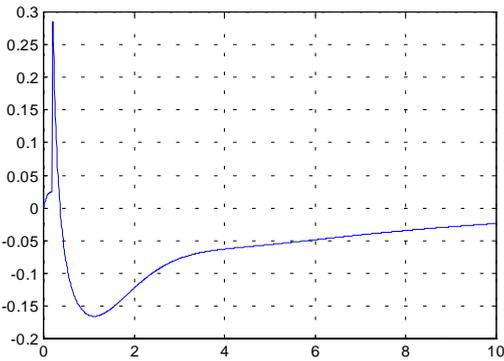
Figure 6 - Control effort ( $\beta$ ) response for a 0.1 step in reference pitch-attitude ( $\theta_{ref}$ ) for the vehicle without the IFD system.
