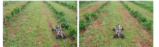
Figure 8. Platform in autonomous mode traversing the orchard corridor. The figure on left and right show the initial vehicle pose and after 10 seconds of execution, respectively.
