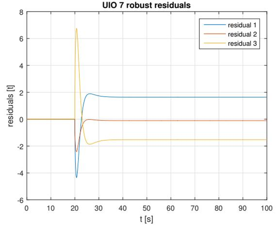
Figure 10. Robust residuals generated from the third UIO of the output bank of observers, which excludes the  $\phi$  angle sensor output.
