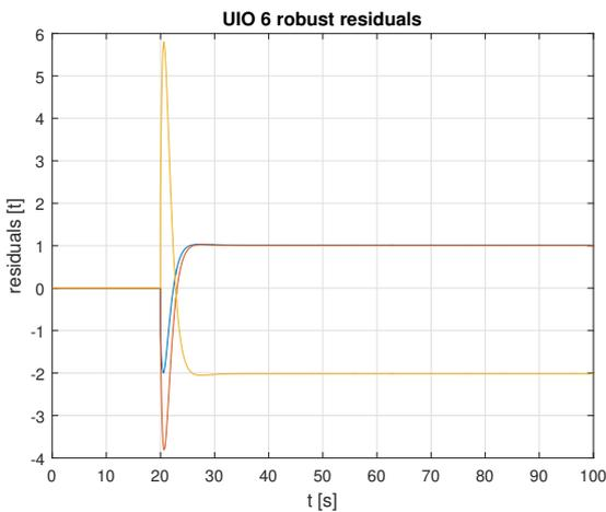
Figure 9. Robust residuals generated from the second UIO of the output bank of observers, which excludes the  $\theta$  angle sensor output.
