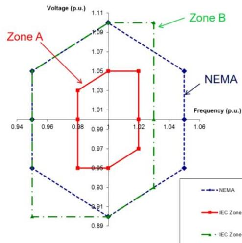
Figure 2. NEMA/IEC Allowable Voltage and Frequency Variations for Motors (NEMA vs. IEC Motor Standards. “Comparison and Contrast of the Two Design Practices,”).
