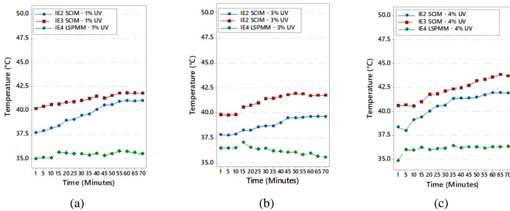
Fig. 8 Temperature rise for undervoltage unbalance conditions for IE2, IE3 & IE4 Class motors with: (a) 1% UV; (b) 3% UV; (c) 4% UV
