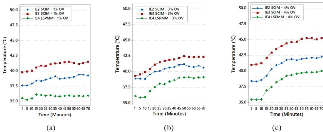
Fig. 9 Temperature rise for overvoltage unbalance conditions for IE2, IE3 & IE4 Class motors with: (a) 1% OV; (b) 3% OV; (c) 4% OV
