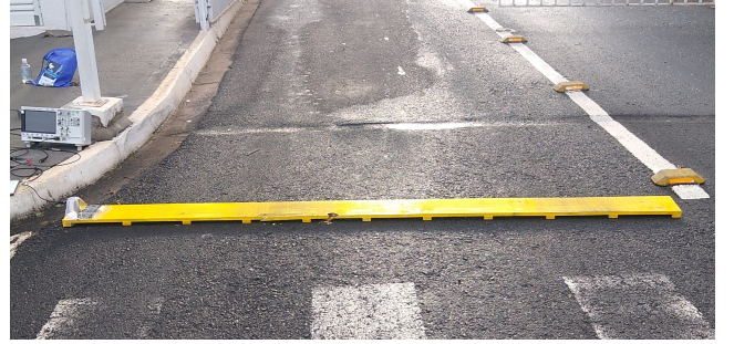
Figure 3. The handmade speed bump with the smartphone docked and positioned to acquire real data.
