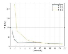
Fig. 17. Measurements of Current and Current THD in the Plant – Sunny Day
