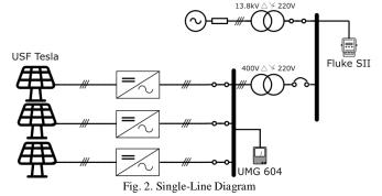
There are three power inverters in the plant: a Jema IF - 15 n (15 kW) - the one that was damaged -, a Fronius IG Plus 150V-3 (10 kW) and a SMA Sunny Tripower 12000TL (12 kW). The power plant has 152 PV panels (Yingli 245P-32b, 245W.) divided in 3 groups that are divided in strings following the detailed scheme below seen in Fig. 3.
