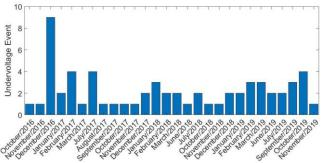
Fig. 11. Number of voltage sag occurrences registered by UMG604
