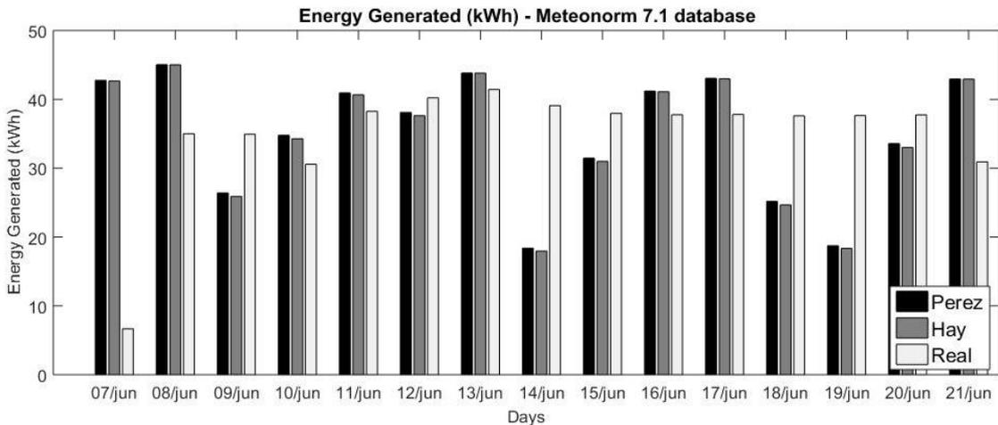
Figure 2: Energy generated (kWh) applying Perez model, Hay model and real data using Meteororm 7.1 meteorological database
