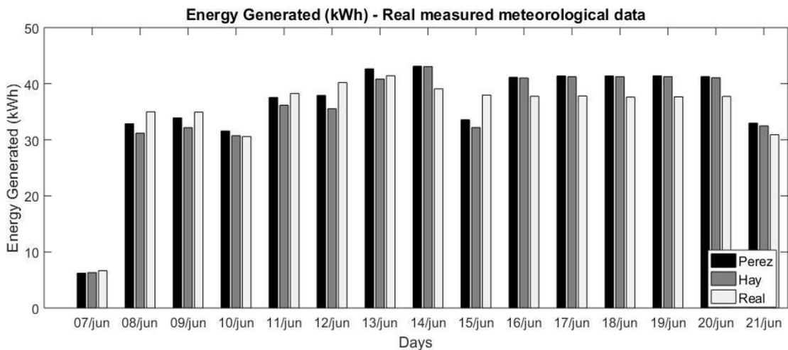
Figure 4: Energy generated (kWh) applying the model of Perez and Hay model using real meteorological data measured on the site.
