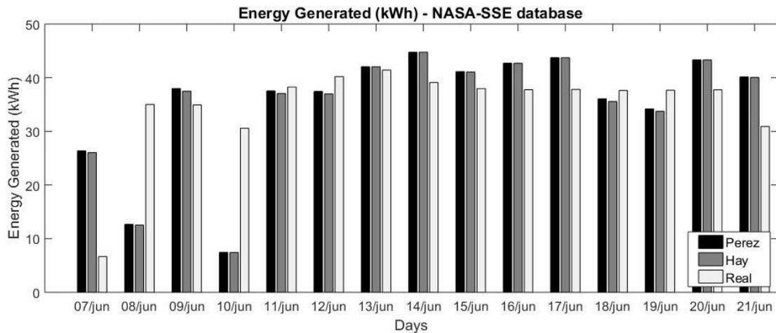
Figure 3: Energy generated (kWh) applying Perez model, Hay model and real data using NASA SSE meteorological database
