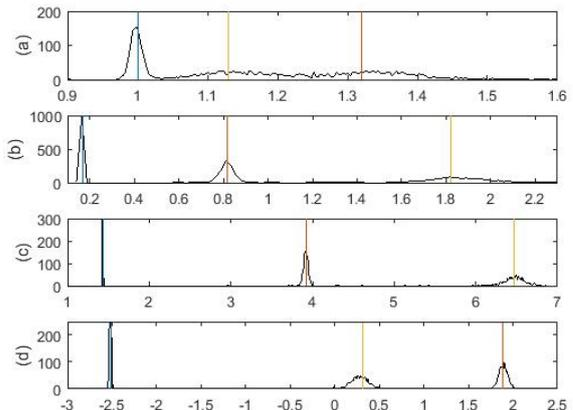
Figure 3: Estimated normalized probability density functions for: (a) amplitude, (b) damping factor, (c) angular frequency and (d) phase. The real values of the parameters are represented by the highlighted constants
