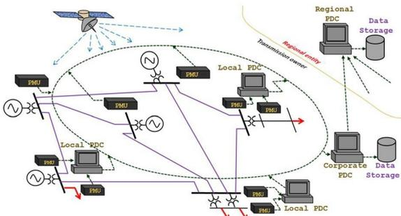
Figure 1: Typical architecture of a wide area synchrophasor network (Annakage et al., 2017).
