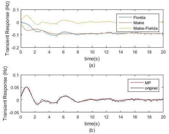
Figure 4: (a) Transient and (b) ringdown response of the NAEI system
