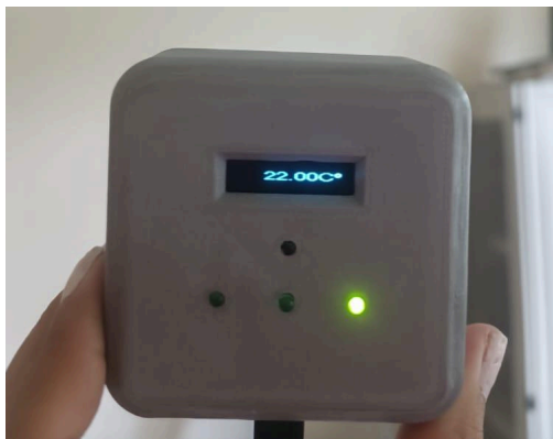
Fig 7. SMAT instalado no Data Center do CEAMAZON.
