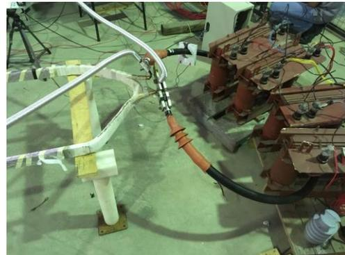
Figure 7. Current induction circuit
