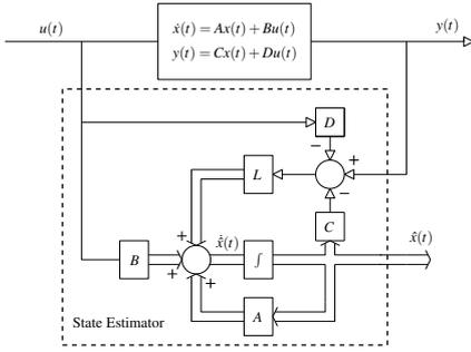
Figure 2: Closed-Loop State Estimator
