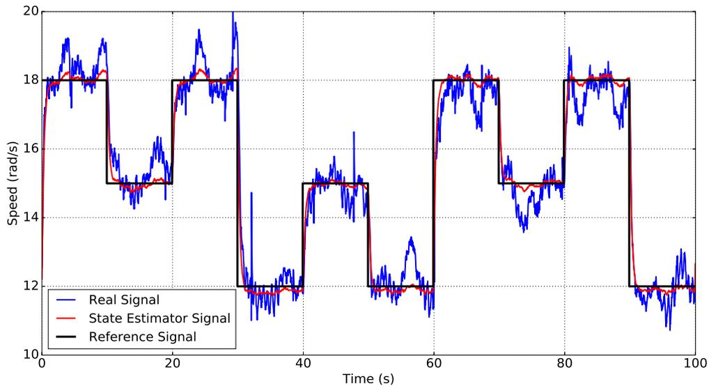
Figure 6: State Estimator Experimental Validation
