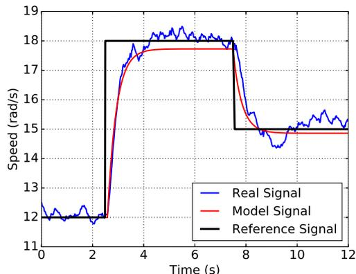
Figure 5: Experimental Model Validation
