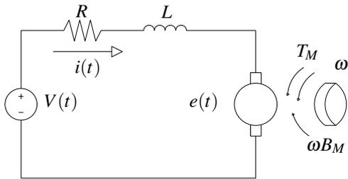
Figure 1: Schematic diagram of the DC motor
