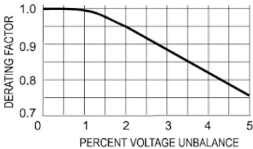
Figure 3. Derating Factor for squirrel cage induction motors due to unbalanced voltage according to NEMA.
