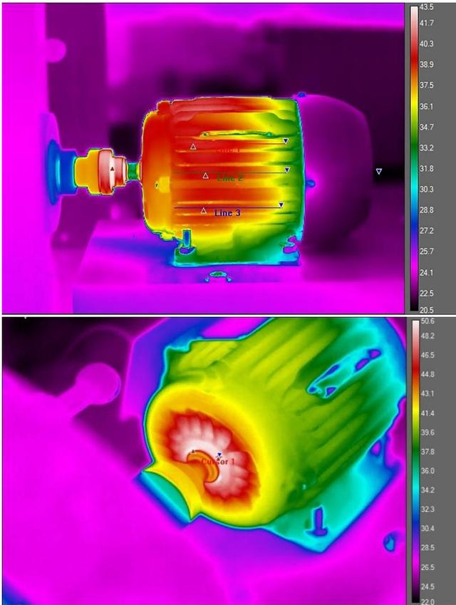
Fig. 5 Thermographic images angles captured for LSPMM.
