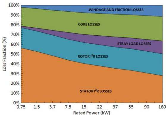
Figure 1. Typical fraction of losses in 50-Hz, four-pole squirrel cage induction motors. (A. T. de Almeida et al., 2014)
