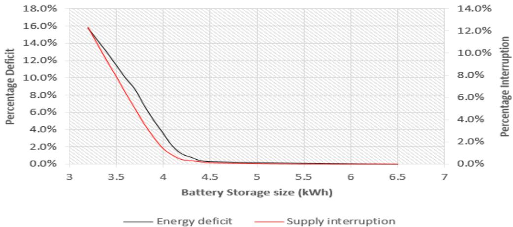
Fig. 6 Energy deficit and supply interruption graphs for the commercial consumer
