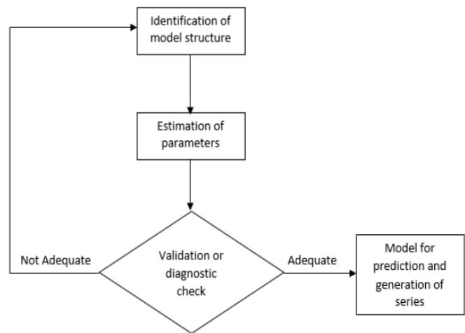
Fig. 1 Flowchart of Box-Jenkins method.
