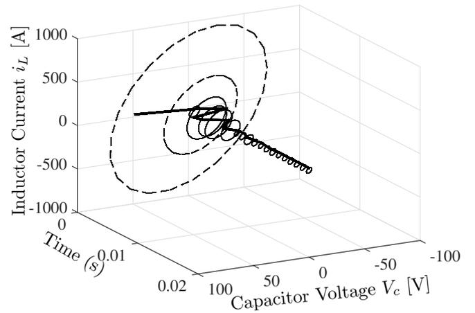
Figure 8. The closed-loop impulse response bounded by ellipsoids in  $x_{set} \times i_L \times V_c$ .
