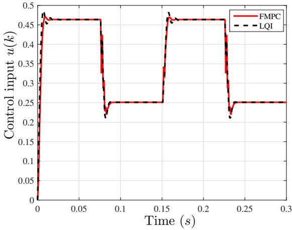
Figure 6. Control signal  $u(k)$ .
