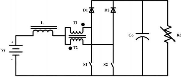
Figure 1. 3SSC Boost Converter (Costa, 2017).
