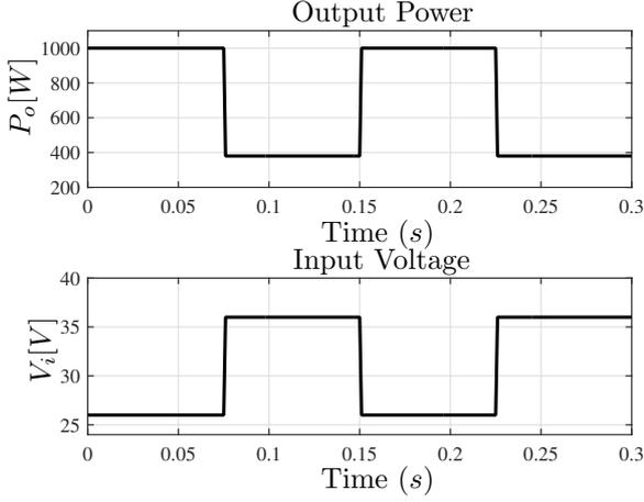
Figure 2. Variation in the operating point of the 3SSC converter.
