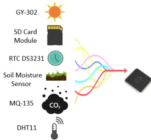
Figure 4. Sensors connections into the microcontroller ATmega 2560.
