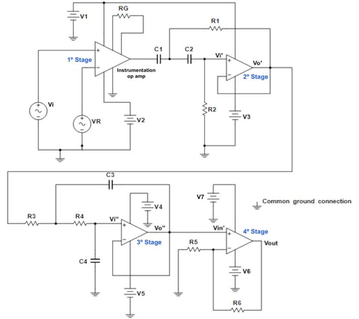
Figure 3. Representation of the developed signal conditioning circuit.
