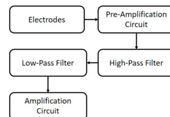
Figure 2. Signal conditioning circuit steps of the electrical signal.
