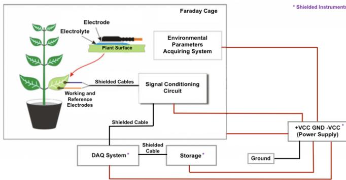
Figure 5. Connections applied in the process of measuring plants electrical signals. Adapted from Cabral et al. (2011).
