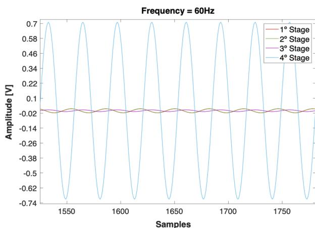
Figure 7. Graphs of each conditioning circuit stage when  $f=60\text{Hz}$ .
