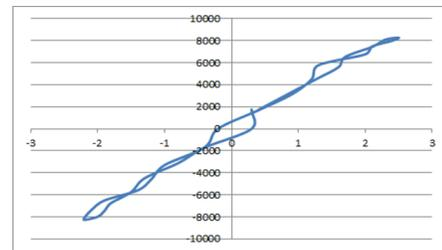
Fig. 8. HIF characteristic curve VxI - Test 2.
