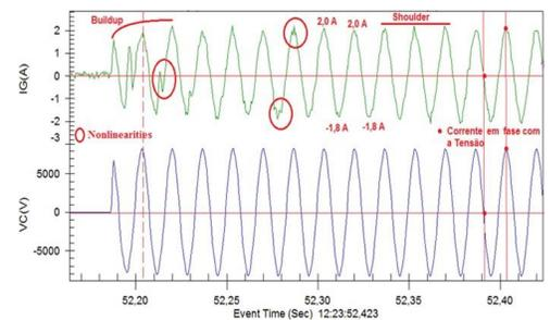
Fig. 11. Details of the HIF chain in Test 3 - Buildup, Shoulder, Nonlinearities and asymmetries.
