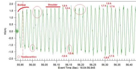
Fig. 13. Details of the HIF chain in Test 4 - Buildup, Shoulder, Nonlinearities and asymmetries.
