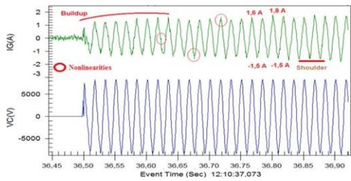
Fig. 9. Details of the HIF chain in Test 2 - Buildup, Shoulder, Nonlinearities and asymmetries.
