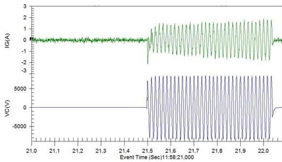
Fig. 5. HIF Current and Voltage of the branch near the cable - Test 1.
