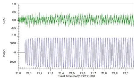
Fig. 14. Current and voltage of HIF of the branch leaning against the cable – representative oscillography of the Tests 5,6 e 7.
