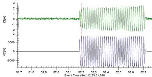
Fig. 10. Current and voltage of HIF of the branch leaning against the cable - Test 3.
