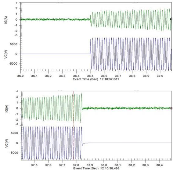
Fig. 7. Current and voltage of HIF of the branch leaning against the cable - Test 2
