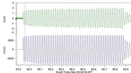
Fig. 12. Current and voltage of HIF of the branch leaning against the cable - Test 4.
