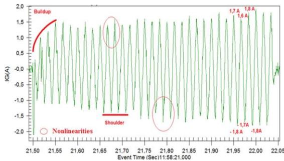
Fig. 6. Details of the HIF chain in Test 1 - Buildup, Shoulder, Nonlinearities and Asymmetries.
