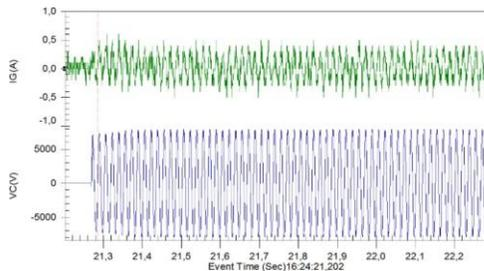
Fig. 15. Current and voltage of HIF of the branch leaning against the cable – representative oscillography of the Tests 8,9 e 10.
