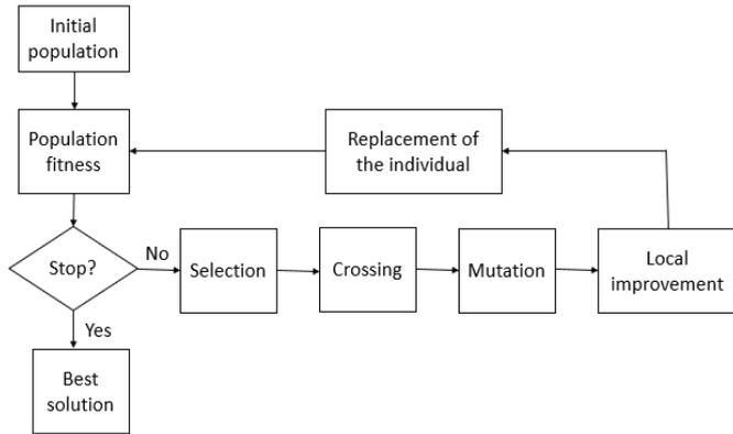
Fig. 3. Flowchart of the optimization algorithm.
