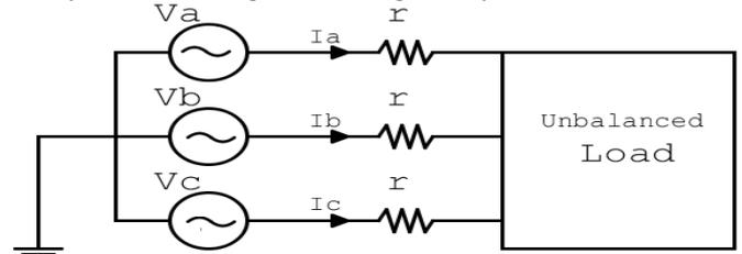
Fig. 1. Unbalanced and symmetrical three-phase system.
