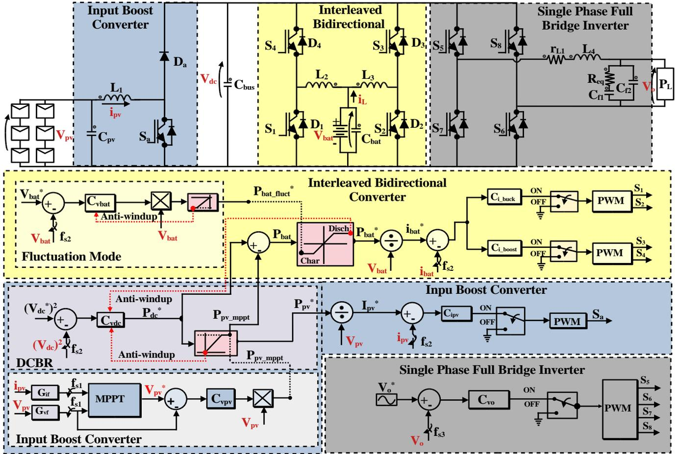
Fig. 3 Block diagram of the proposed control strategy for the off-grid PV system.
