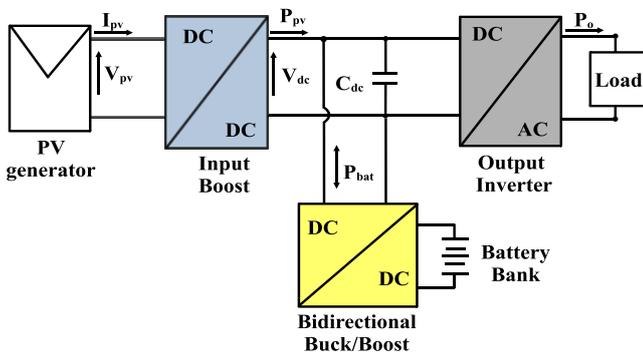
Fig. 1 Off-grid PV system
