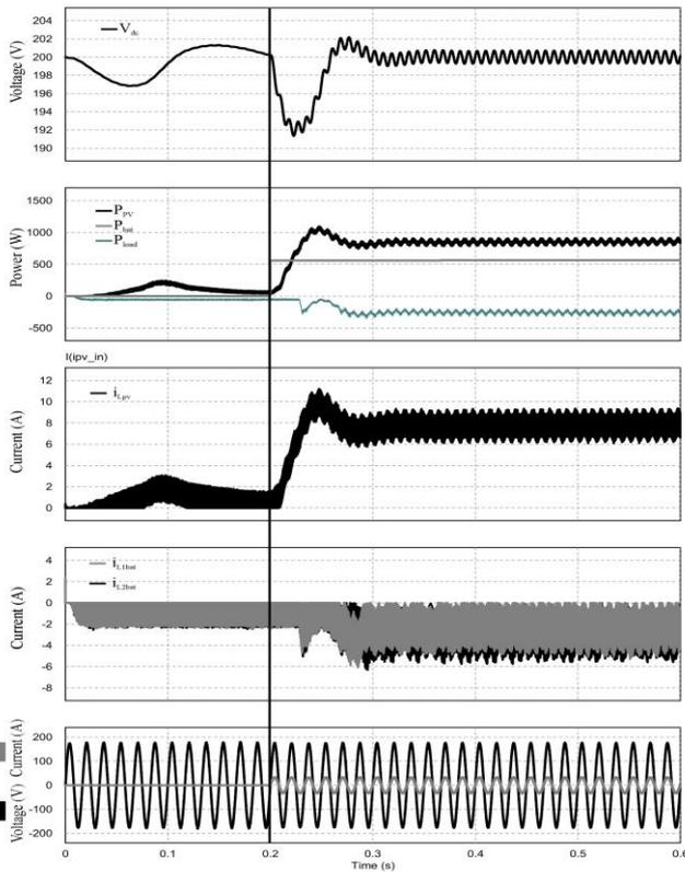
Fig. 4 Simulation results for Buck mode operation under load variation.
