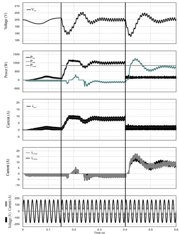
Fig. 6 Simulation results for transition modes from Buck to Boost modes under loads and irradiation variations
