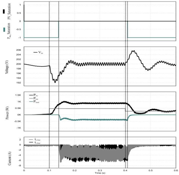
Fig. 5 Simulation results shows both saturations of the system under loads variation while operating in Buck.
