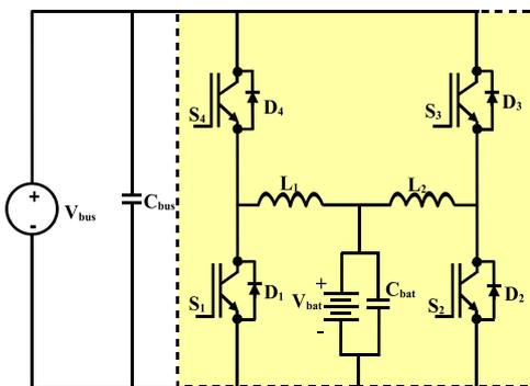
Fig. 2 Interleaved battery-bank converter interface with two power modules.
